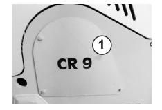
Remove the left side cover (1) as viewed from the guide bar. Open the maintenance cover (2) (fold forward).
