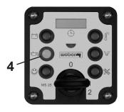
Charge level LED (5) is illuminated. Charging voltage too low or not available. Battery is not being charged. Engine does not switch off.
