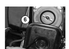
Remove the air filter insert (7) from the air filter enclosure. Clean air filter insert as specified by the engine manufacturer if there is damage or if it is extremely dirty.
