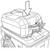
▶ Push the battery pack down and hook in the battery fastener.
