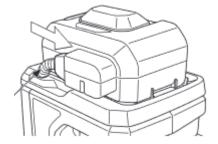
► Remove the protective cap from the battery connector and insert the power cable.
