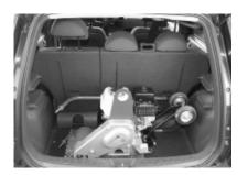
For transport in a vehicle, the guide bar (2) can be removed. To do this, remove the safety cotter (3) and pull the guide bar (2) out of the holder.
