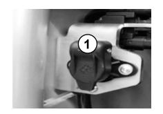
Insert plug (1) into the charging socket.
