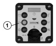
Charge level LED (1) is illuminated. Charging voltage too low or not available. Battery is not being charged.
