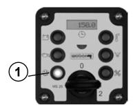
Oil pressure indicator (1) is illuminated. Oil level too low. Engine shuts down immediately. Error must be corrected prior to restart.
