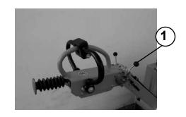
Push the parking brake lever (1) into vertical position (disengage).
