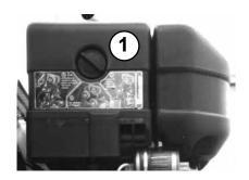
Remove the air filter insert (1) from the air filter enclosure. Clean air filter insert as specified by the engine manufacturer if there is damage or if it is extremely dirty.
