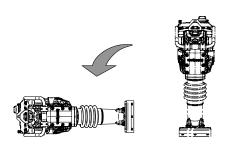
ATTENTION! If the tamper is laid down on the side with the air filter, residual gasoline may enter the air filter. This may cause damage to the air filter.
