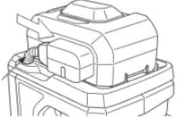
Tip the battery back and insert the claw into the battery hook.
