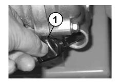
Remove the oil drain screw (1) and drain oil.
