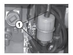
► Drain the fuel tank into a suitable clean vessel.
