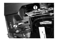
Turn the short-circuit button to the "0" - OFF position.
