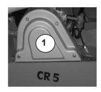
Check the V-belt (1) for cracks, damaged flanks, and wear.
