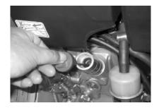
Checking the engine oil level
