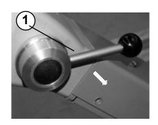
Control drive speed and direction of travel with the handle (1).
