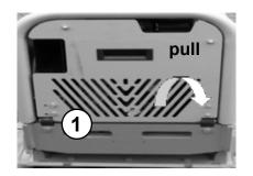
Pull the oil dip stick (1) out of the crankcase.
