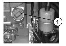
Screw the oil drain pipe (1) onto the engine drain valve and drain off the oil.
