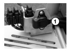
Insert plug (1) into the charging socket.
