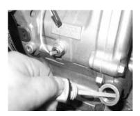
The correct oil level is between the min. and max. marks.
