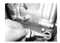
Screw the oil drain pipe (1) onto the engine drain valve and drain off the oil.
