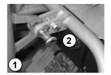
Fit the crane hook into the hinged lifting ring (1) and lift the machine onto the desired means of transport.
