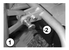
Mount the retaining pin (1) on the base plate.
