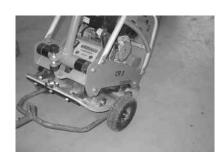
Engage the retaining pin (1) in the retaining element (2) of the undercarriage.
