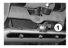
Slide the hand truck under the base plate.
