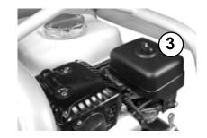
Remove the air filter insert (4) from the air filter enclosure. Clean air filter insert as specified by the engine manufacturer if there is damage or if it is extremely dirty.
