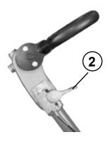
Turn the short-circuit button (3) to the "1" – ON – position.
