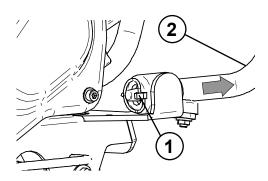
The guide bar can be removed for transport. This makes it possible to transport the machine, e.g. in the trunk of a car.
