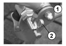
Use the two screws (2) to fasten the undercarriage (1) at the engine bracket.
