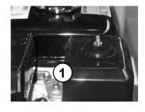
Remove the air filter (1) insert from the air filter enclosure Clean the air filter insert in accordance with theguidelines provided by the engine manufacturer, or replace if there is extreme fouling.
