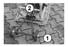
Use the handle (1) to tilt the machine to the front and swivel the undercarriage (2) beneath the base plate (3).
