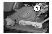
Check the V-belt (1) for cracks, damaged flanks, and wear.
