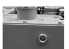
Check the hydraulic fluid level in the view glass (1).
