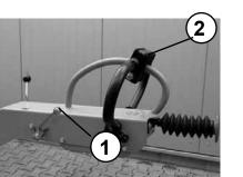
Turn the ignition key (1) from position  $_{,l}$ " to position  $_{,0}$ ". Pull out the ignition key.
