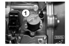
Screw the oil drain pipe (1) onto the engine drain valve and drain off the oil.
