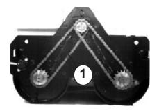
Loosen the fastening screws (1) of the hydraulic motor to tighten the chains.
