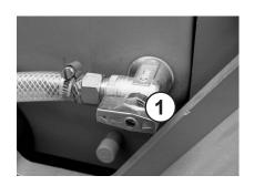
Push the stop lever (1) of the engine to the left.
