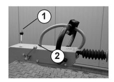
Insert the ignition key (1) and turn to position 1. Turn the ignition key (1) to position 2.
