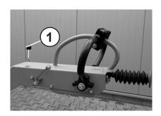
Push the parking brake (1) into vertical position (disengage).
