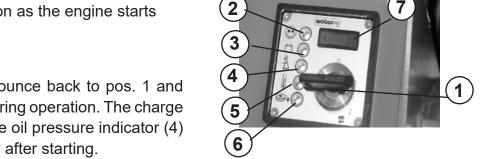
The ignition key must bounce back to pos. 1 and remain in this position during operation. The charge level indicator (3) and the oil pressure indicator (4) must go out immediately after starting.
