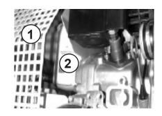
Top up hydraulic liquid. Check the hydraulic fluid level in the view glass (1).
