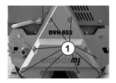
Lubricate the chains (1) as needed and in accordance with the specification.
