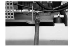
After emptying completely, unscrew the oil drain pipe from the drain valve and fill with oil in accordance with the specification.
