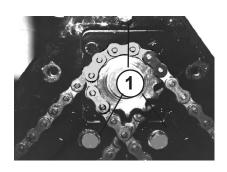
Lift hydraulic motor (1) until the chains (2) have reached the desired tension.
