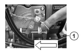
Turn the ignition key (1) from position "I" to position "0". Pull out the ignition key.
