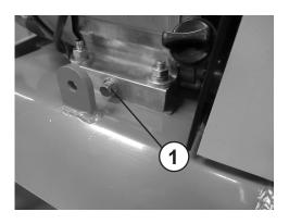
Remove the oil drain plug (1)
