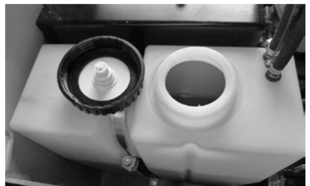
► Check the hydraulic oil level using the view glass (4).
