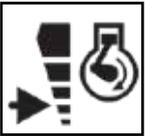
The engine speed selector switch switches ECO mode on or off.
