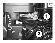
Turn the short-circuit button (1) to the "0" - OFF position.
