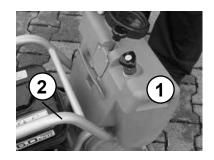
Star screw (1) down press and tank mounted in the frame (2).
