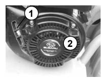
After the engine has warmed up, slide the choke lever (2) to the right (open).
