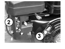
After the engine has warmed up, slide the choke lever (2) to the right (open).
