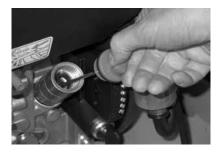
The correct oil level is between the min. and max. marks.
