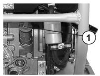
Screw the oil drain pipe (2) onto the drain valve and drain the oil.
