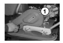
Check the V-belt (1) for cracks, damaged flanks, and wear.
