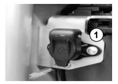
Insert plug into the charging socket.
