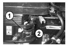
Slowly tighten the handle (1) of the reversing starter (2) until resistance is noticeable.
