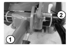
Unlock the retaining pin (1).
