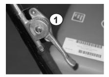
Unlock the cutting depth adjustment lever (1) and set desired cutting depth.
