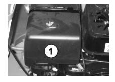
Remove the air filter insert (1) from the air filter enclosure.
