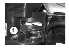
Turn the short-circuit button to the "0" – OFF-position.
