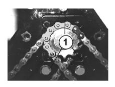
Lift hydraulic motor (1) until the chains (2) have reached the desired tension.
