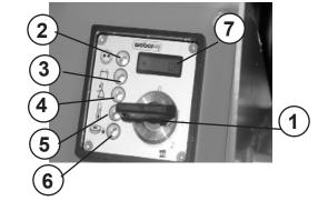
The ignition key must bounce back to pos. 1 and remain in this position during operation. The charge level indicator (3) and the oil pressure indicator (4) must go out immediately after starting.
