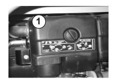
Remove the air filter insert (1) from the air filter enclosure. Clean air filter insert as specified by the engine manufacturer if there is damage or if it is extremely dirty.
