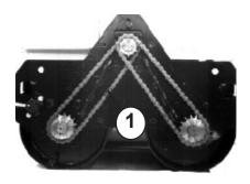
Loosen the fastening screws (1) of the hydraulic motor to tighten the chains.
