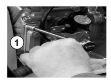
Replace oil filter (1) with a new element. After replacing the filter element, seal the filter enclosure with the cover cap.
