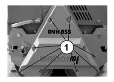
Lubricate the chains (1) as needed and in accordance with the specification.
