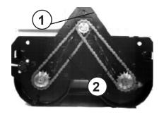
Check/tighten drive chains Remove the chain guard (1).
