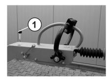
Push the parking brake (1) into vertical position (disengage).
