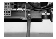
After emptying completely, unscrew the oil drain pipe from the drain valve and fill with oil in accordance with the specification.
