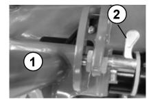
Fit the crane hook into the ring (1) and lift the machine onto the desired means of transport.
